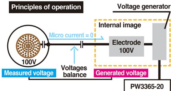
Inside the PW9020 is an electrode (a metal plate). When there is a potential difference between this electrode and the measured line, a minute current flows as a result. By detecting this minute current and generating a voltage such that the current declines to zero, it is possible to accurately measure the voltage without being affected by the outer diameter of the measured cable or its insulation.
