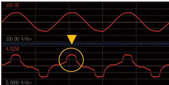
Current flows only near the peak of the voltage waveform
