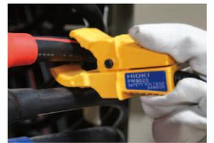
STEP4 Connect the clamp sensors
