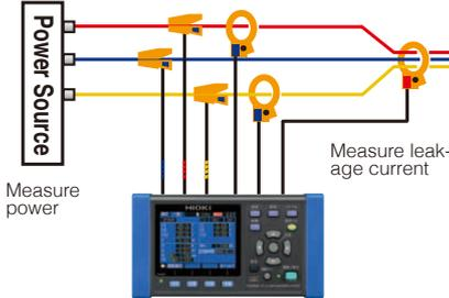
With the ability to calculate and process data every 200ms, you can do simple checks of intermittent leakage current. Choose from average, maximum and/or minimum value of the measured interval.
