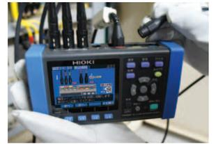
STEP3 Connect the voltage sensor
