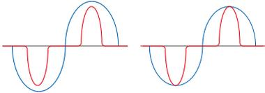
Current flows only near the peak of the voltage waveform, resulting in a voltage drop that flattens the peak portion of the voltage waveform.
