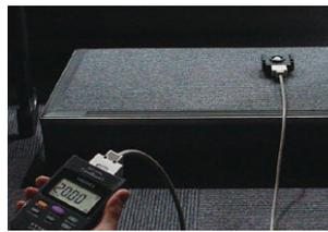
Sensor unit and main display can be separated to 2m, letting you measure at a distance away from the sensor in order to accommodate for difficult locations, shadows, and other issues.
