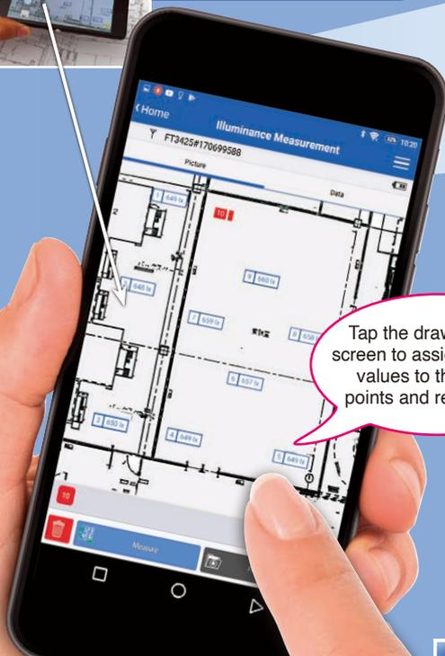
Tap the drawing on the screen to assign measured values to the desired points and record them.
