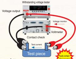
◆ If a test lead were to come lose during testing with a measurement device that does not offer contact check functionality, defective test pieces would be judged to be non-defective.
