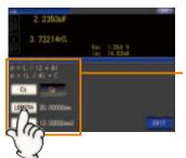
Enter the following parameters: Conductor length (LENGTH) Conductor cross-sectional area (AREA)
