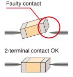
The Hi-Z reject function outputs an error if the measurement result exceeds a preset judgment standard. This capability enables the instrument to detect poor contact when performing measurement using a two-terminal fixture.
