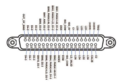
Signal assignment is different during continuous measurement mode. Signal logic is 0 V to 0.9 V for LO level and 5 V to 24 V for HI level.
