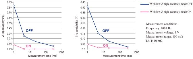
Low-Z high-accuracy mode can be used with the 100 m $\Omega$ , 1  $\Omega$ , and 10  $\Omega$  ranges.
