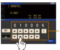
The judgment standard is calculated based on the measurement range and judgment reference value (valid setting range: 0% to 30,000%).
