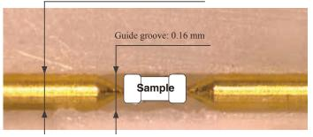
Shape of probe tip: 60° cone
