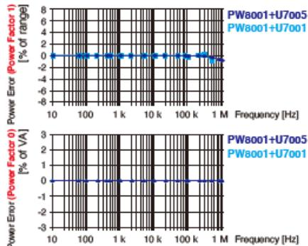
The PW8001 measures even high-frequency and low-power-factor power with a high degree of accuracy
