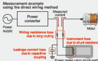
The wiring of the measurement target is routed for connecting to the current input terminal. However, this results in an increase in the influence of power loss from wiring resistance and capacitive coupling, and meter loss due to shunt resistance. All of this loss leads to larger degradation in accuracy.
