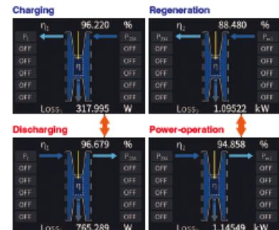
PW8001 detects charging/discharging and power-operation/regeneration states and switches the direction of energy flows automatically.
