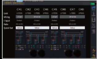
Use the connection confirmation screen to prevent wiring mistakes.
