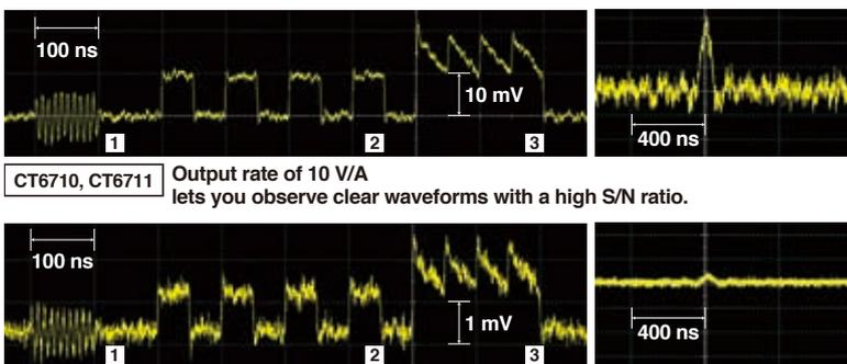
**CT6710, CT6711** Output rate of 10 V/A lets you observe clear waveforms with a high S/N ratio.
