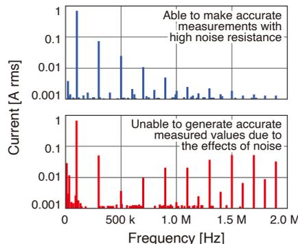
For reactors, higher frequencies mean lower current values. The image to the right shows a waveform obtained by measuring reactor current at high frequency along with variations in current values that accompany variations in the frequency.
