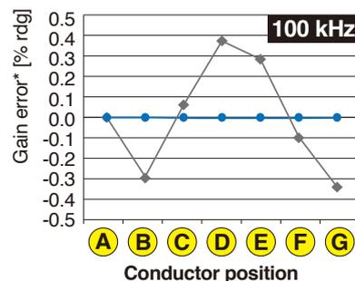
— CT6904A — Sensors designed without accounting for conductor position
