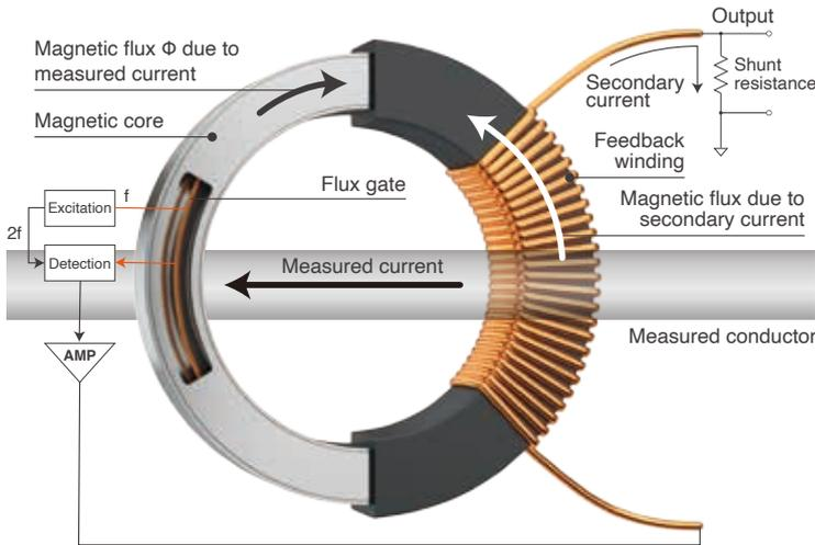
High-frequency currents are detected by a winding (CT), while DC to low-frequency currents are detected by a flux gate.
