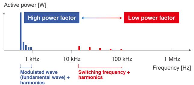
Since the power factor decreases with harmonics, current sensors' phase measurement accuracy becomes key (see right).
