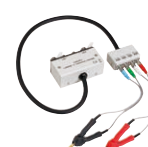
4-TERMINAL PROBE L2000 Ideal for clipping to screw terminal, cable length of 1 m (3.28 ft.), cannot be used with 3 mΩ range when connected to BT4560, no combined accuracy defined
